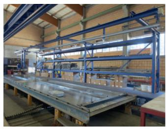
Afterwards: On the left the new state-of-the-art storage, cleaning and plotting device with new controller. On the right the manual shuttering station in the form of the workplace system with mobile tool trolley, hot-glue gun, manual oiler, rack system and gangway alongside the pallet. Control consoles for pallet movement directly adjacent to the work station. On the pallet is fresh shuttering with integrated magnets.
