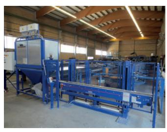
Afterwards: Shuttering transport with cleaner/oiler for shuttering with integrated magnets. Automatic cleaning/oiling of the shuttering and transport of the shuttering from the demoulding station direct to the shuttering station.
