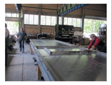
Previously: Shuttering and magnets separate, storage of the shuttering parts and built-in components as well as tools such as glue gun, etc. took place from the front side of the pallet, hence long distances. Manual cleaning of the shuttering and magnets.
