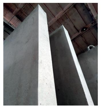
Weckenmann developed a semi-mobile battery formwork version with increased structural strength for the customer. All elements of a prefabricated apartment building can be manufactured in this single battery formwork - including solid floor slabs up to a thickness of 180-200 mm.
