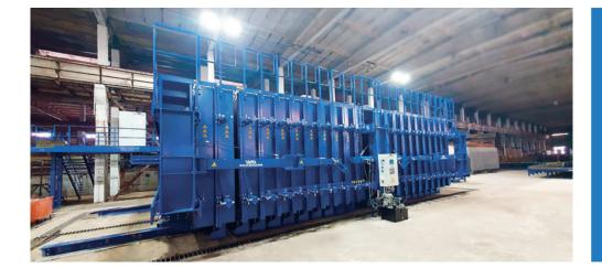
One battery formwork unit covers Tetra's entire extensive product range of different sized precast elements.
